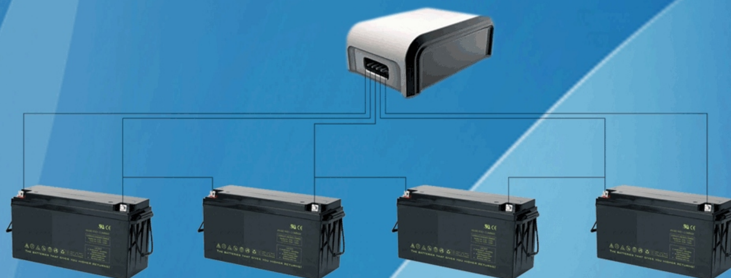
CONNECTION DIAGRAM SHOWING FOUR BATTERIES BEING EQUALIZED BY BATTERY EQUALIZER
